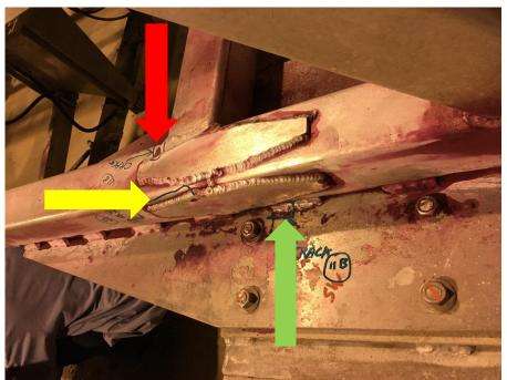
Photo of area 11B Red arrow shows location of crack in parent material yellow arrow shows lack of fusion on fish plate weld and green arrow shows crack on stitch weld. All at location
