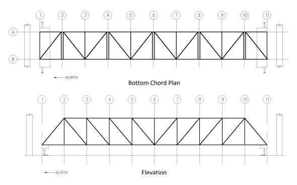
Figure 1: Bridge Collector Plan & Elevation
