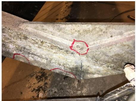
Photo showing pitted corrosion in scum paddle arm This is typical to all below water line aluminum members
