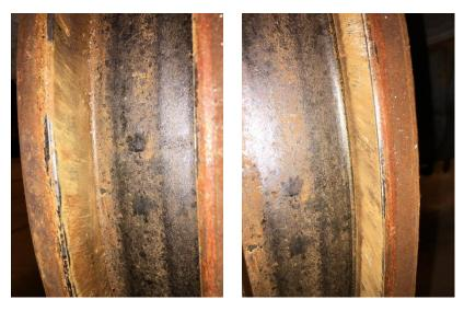
Figure 6: Wear on North End-Truck Wheels
